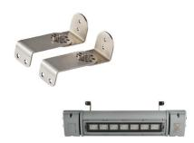
The Nemalux Swivel Bracket Mounting Kit is designed for ceiling and wall mounting of all Nemalux Linear luminaires. There is the facility to rotate the fitting through various angles to suit any application. The stainless-steel bracket provides lock-in holes every 30° and 45°. Shorter length variants are available providing part-rotation for restricted space applications.
