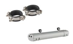
The Nemalux Pole Clamp Kit is designed to pole-mount any Nemalux Linear unit. The stainless-steel circular brackets are provided in a pair and easily screw to the back of the Linear unit, with adjustable side-bolts to open and clamp around a single pole. Kits to suit poles up to 62mm in diameter are available.
