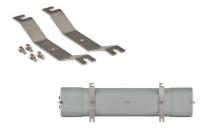
The Nemalux Ceiling Mount Kit is designed to mount to any flat serface, both ceiling and wall. Provided in a pair, two low-profile stainless-steel U brackets screw easily to the back of the Linear unit, then onto the chosen surface. 1000mm and 1500mm variants.
